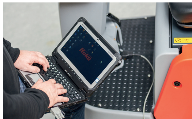
Easy access to the diagnosis interface for maintenance purposes and to modify machine settings.
